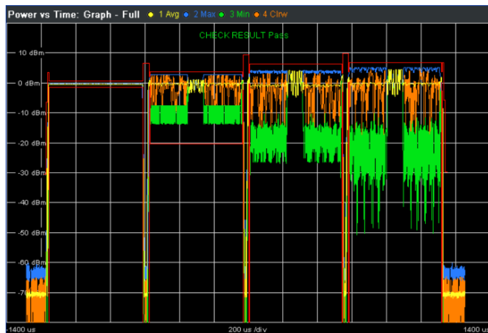
Fig. 2-8: Full Burst view in Power vs Time
